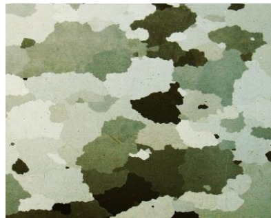
Figure 4. Grain-oriented electrical steel without coating showing the polycrystalline structure. Image 6.0 x 4.8 cm. © Zureks 2007, Wikipedia
